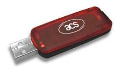
The ACR38T is a stylish plug-in (SIM-sized) smart card reader/writer. It has the full functionalities of ACR38 and supports smart cards that conform to GSM 11.11 specification.
